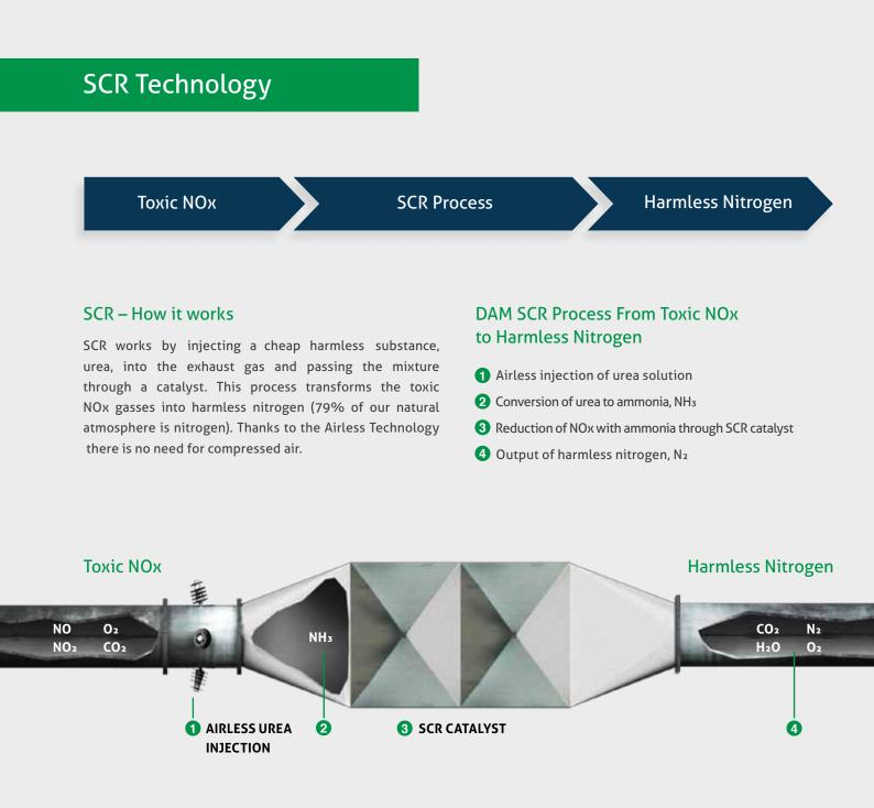
The Digital Airless Multipoint SCR process from toxic NOx to harmless nitrogen
